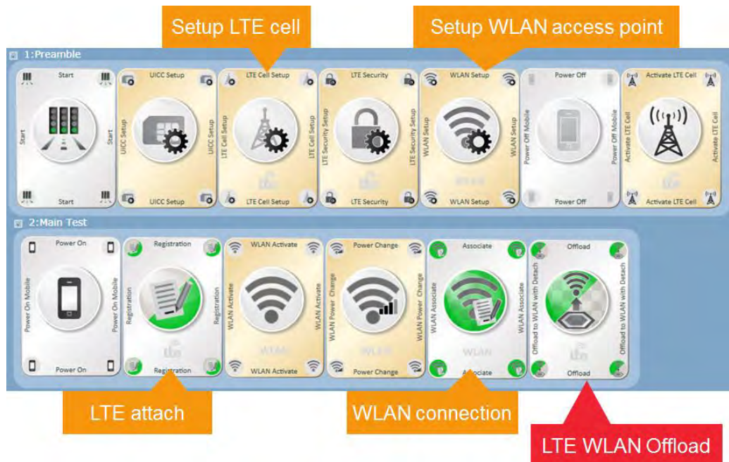
Fig. 3-32: CMWcards Example for Release 12: LTE-WLAN Offloading.
