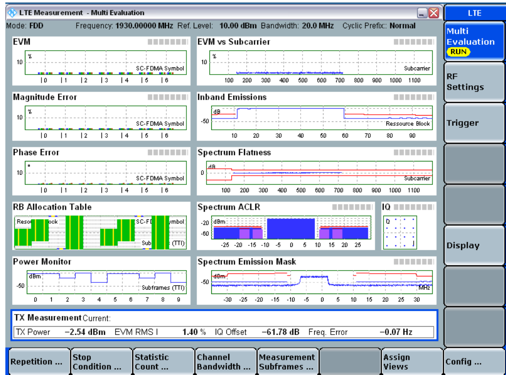
Fig. 3-34: Tx measurements of a DUT uplink signal using CMW500.
